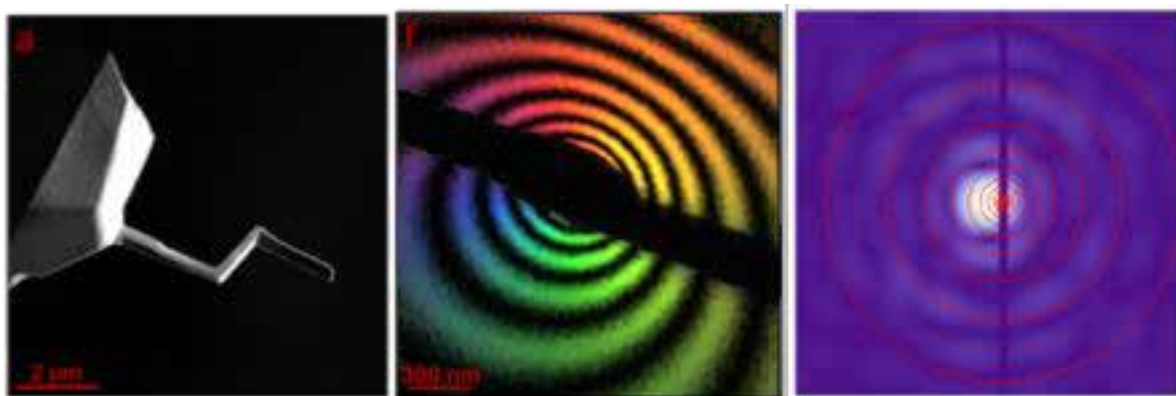
Fig. 1 Left: SEM view of part of the TAPP device; the central segment of the wire is positioned parallel to the electron beam, and current is injected into it after establishing electrical contact. Center: contour map of the TAPP phase shift; the asymmetry of the contours is due to the perturbed reference wave, but does not affect the operation of the device. Right: calculated TAPP phase shift superimposed to the shadow of the wire and to the spectrum of a phase object corresponding to a biomolecular complex.
